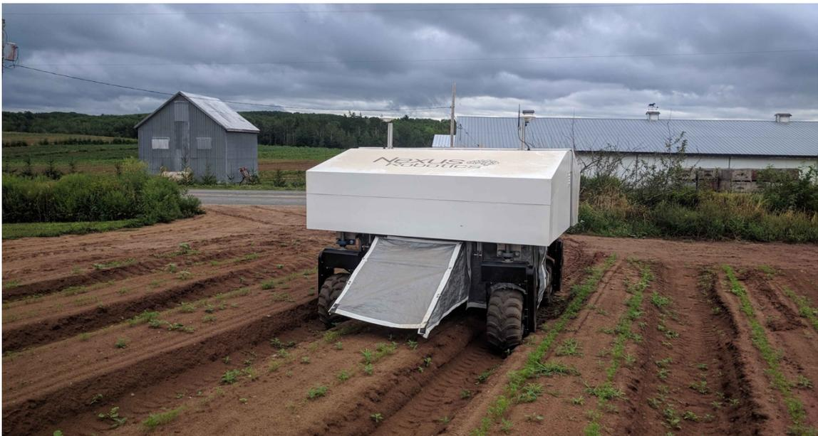
**Figure 1.1: Nexus Robotics autonomous weeding robot “R2-WEED2”. [1]**
